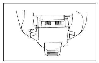
Your vehicle is equipped with a seven-wire trailer towing harness. This harness has a seven-pin universal heavy-duty trailer connector (if equipped with the trailering package) that is attached to a bracket on the hitch platform. If your vehicle is not equipped with the heavy-duty trailer connector, you may purchase one from your dealer. The seven-wire harness contains the following trailer circuits:
