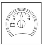
When your engine is not running, but the ignition is in RUN, this gage shows your battery's state of charge in DC volts.
