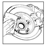
8. Remove any rust or dirt from the wheel bolts, mounting surfaces, and spare wheel.
