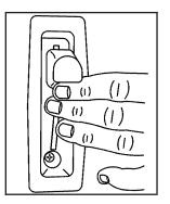
2. Lift the lever, located on the outboard side of the seatback, and fold the seatback forward.
