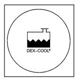
The engine coolant recovery tank is in the engine compartment on the passenger's side of the vehicle. The cap has this symbol on it. See *Engine Compartment Overview on page 366* for more information on location.
