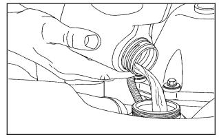
3. Fill the radiator with the proper DEX-COOL<sup>®</sup> coolant mixture, up to the base of the filler neck. See *Engine Coolant on page 379* for more information about the proper coolant mixture.
