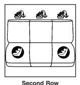
(Top Tether Anchor): Seating positions with top tether anchors.
