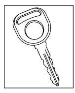
This vehicle has keys that can be used for the ignition and door lock that will fit with either side up.
