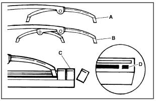
To install the new wiper insert, slide the insert (D), notched end last, into the end with two blade claws (A). Slide the insert all the way through the blade claws at the opposite end (B). The plastic caps (C) will be forced off as the insert is fully inserted. 5. Be sure that the notches are locked by the bottom claws. Make sure that all other claws are properly locked on both sides of the insert slots.
