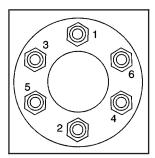
13. Use the wrench to tighten the wheel nuts firmly in a crisscross sequence as shown.
