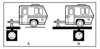
The trailer tongue weight (A) should be 10 percent to 15 percent of the total loaded trailer weight, up to a maximum or 400 lbs (181 kg) with a weight carrying hitch. The trailer tongue weight (A) should be 10 to 15 percent of the total loaded trailer weight, up to a maximum of 750 lbs (340 kg) with a weight distributing hitch.
