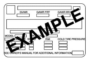
A vehicle specific Certification/Tire label is found on the rear edge of the driver's door. The label shows the size of your vehicle's original tires and the inflation pressures needed to obtain the gross weight capacity of your vehicle. This is called Gross Vehicle Weight Rating (GVWR). The GVWR includes the weight of the vehicle, all occupants, fuel, cargo, and trailer tongue weight, if pulling a trailer.
