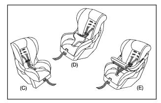
A rear-facing infant seat (B) provides restraint with the seating surface against the back of the infant. The harness system holds the infant in place and, in a crash, acts to keep the infant positioned in the restraint. A forward-facing child seat (C-E) provides restraint for the child's body with the harness and also sometimes with surfaces such as T-shaped or shelf-like shields.
