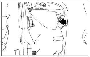
To get an accurate reading, the vehicle should be on a level surface. If the level is below the bottom of the filler plug hole, located on the front axle, you may need to add some lubricant.
