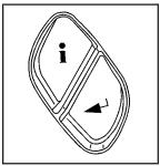
**(Trip Information):** Press this button to display the odometer, trip odometers, and timer.
