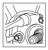
Using the wheel wrench, loosen all the wheel nuts. Do not remove them yet.
