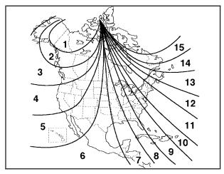
Press and hold the on/off button for six seconds. Release the button when (FOR ZONE) is displayed. The number shown is the current zone number. 3. Scroll through the zone numbers that appear in the window on the mirror by pressing the on/off button. Once you find your zone number, release the button. After about four seconds, the mirror will return to the compass display, and the new zone number will be set.
