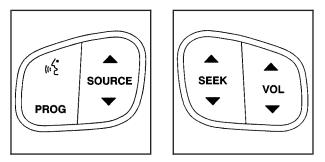
If your vehicle has this feature, some audio functions can be adjusted at the steering wheel. They include the following:
