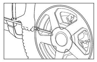
1. If your vehicle has a wheel cap that covers the wheel nuts, position the chisel end of the wheel wrench in the notch and pry it off.
