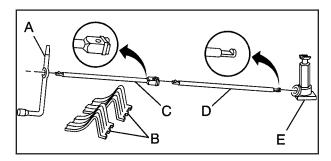
The tools you will be using include the wheel wrench (A), wheel blocks (B), extension(s), (socket end) (C), handle (jack end) (D), and jack (E).
