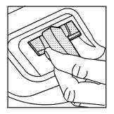
The tilt lever is located to the left of the steering column, under the turn signal lever.
