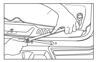
4. Turn the wheel wrench counterclockwise to lower the spare tire. Keep turning the wheel wrench until the spare tire can be pulled out from under the vehicle.
