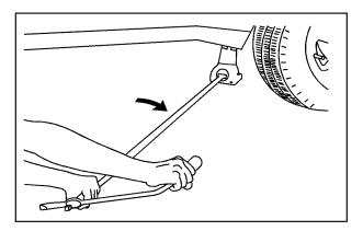
6. Raise the vehicle by turning the jack handle clockwise. Raise the vehicle far enough off the ground so there is enough room for the spare tire to fit.
