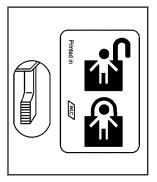
Move the lever down to engage the security lock. Move the lever up to disengage the security lock. The rear doors of your vehicle cannot be opened from the inside while this feature is in use. If you want to open the rear door while the security lock is on, unlock the door and open the door from the outside.
