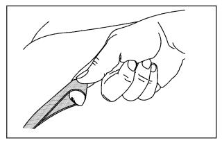
1. Pull up on the loop located where the seat cushion meets the seatback and flip the seat cushion forward.
