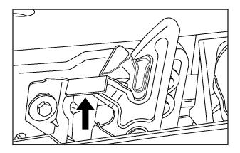
Before closing the hood, be sure all the filler caps are on properly. Then lift the hood to relieve pressure on the prop rod. Remove the prop rod from its slot in the hood and return the prop to its retainer. Lower the hood 6 to 8 inches (15 to 20 cm) above the vehicle and release it to latch fully. Check to make sure the hood is closed and repeat the process if necessary.
