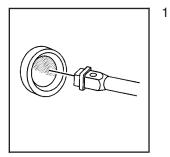
11. If the spare tire is hanging from the cable, insert the socket end of the extension into the hoist shaft hole on a 45 degree angle downward. 12. Be sure that the socket end of the extension connects to the hoist shaft.
