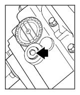
To get an accurate reading, the vehicle should be on a level surface. If the level is below the bottom of the filler plug hole, located on the transfer case, you'll need to add some lubricant. Add enough lubricant to raise the level to the bottom of the filler plug hole. Use care not to overtighten the plug.
