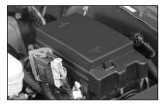
The fuse block is located under the hood in the engine compartment on the driver's side of the vehicle. See *Engine Compartment Overview on page 366* for more information on location.
