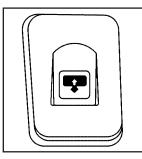
Press and release the back of the control in the overhead console to open the sunroof. Press the front of the control to close the sunroof.
