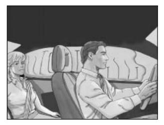
If your vehicle has a roof-mounted airbag for the driver and the person seated directly behind the driver, it is located in the ceiling above the side windows.
