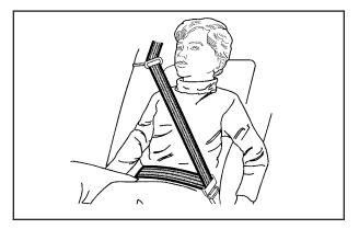
4. Buckle, position, and release the safety belt as described in *Rear Seat Passengers on page 33*. Make sure that the shoulder belt crosses the shoulder.
