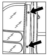
2. Remove the two screws from the taillamp assembly.
