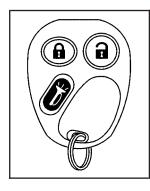
**a** (Unlock): When you press unlock, the driver's door will unlock automatically, the parking lamps may flash and the interior lights will go on.
